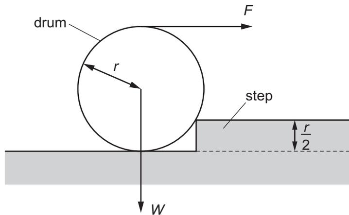
What is the minimum force  $F$  required for the drum to start rolling on the step?
