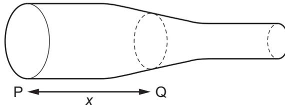
The resistance  $R$  of the wire is measured between end P and Q, a distance  $x$  from P.
