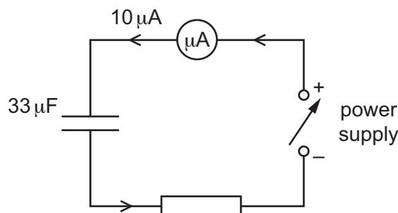
The capacitor is initially uncharged. The voltage across the power supply is then varied so that a current of  $10\ \mu\text{A}$  flows for  $5.0\ \text{s}$ .
